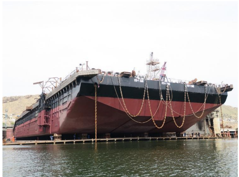
Purpose-built jacket transportation and launch barge, STB-1
