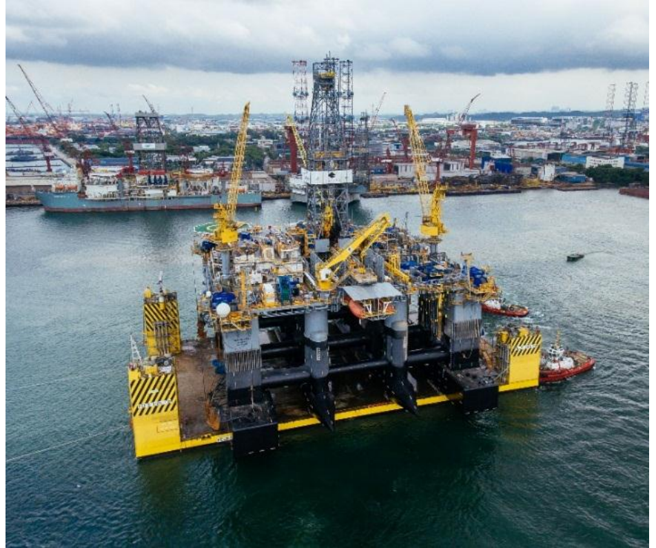
Refurbishment of semi, Ocean Apex
