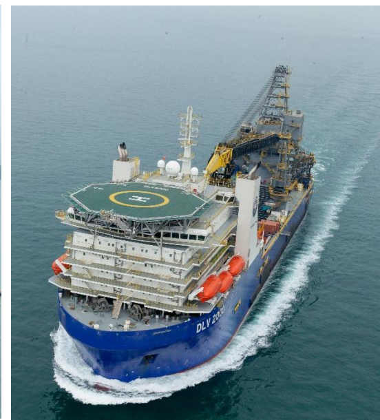
Derrick lay vessel, DLV 2000
