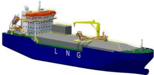
8,000/10,000 cbm Bunker Vessel Max. Draft: 4.8 - 6m
