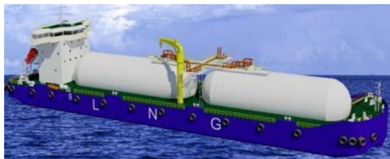
12,000 cbm Shuttle Barge Max. Draft: 3.5m
