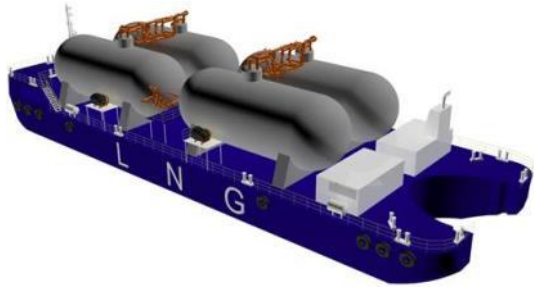
3,000 cbm Non-Propelled Barge Max. Draft: 3.8m
